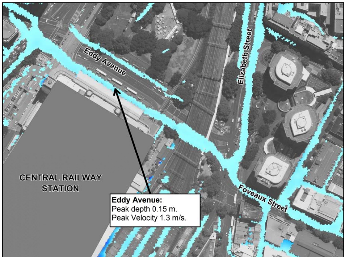
Figure 5-13 Peak flood depths at Eddy Avenue near Central Railway Station
